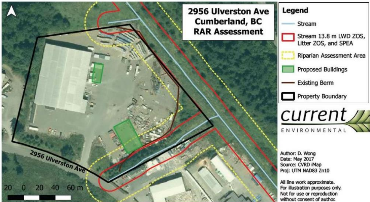
Figure 2. Site plan showing the watercourses affecting the proposed development at the subject property.
