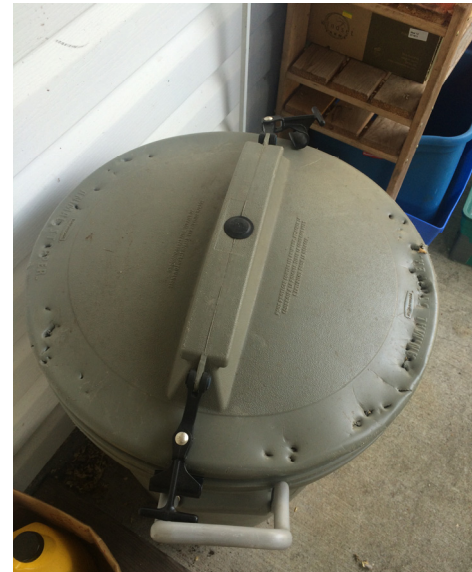
Figure 33. Example of Non Bear Resistant Bin with Bear Damage Fall 2018, Taken on 7th Street
