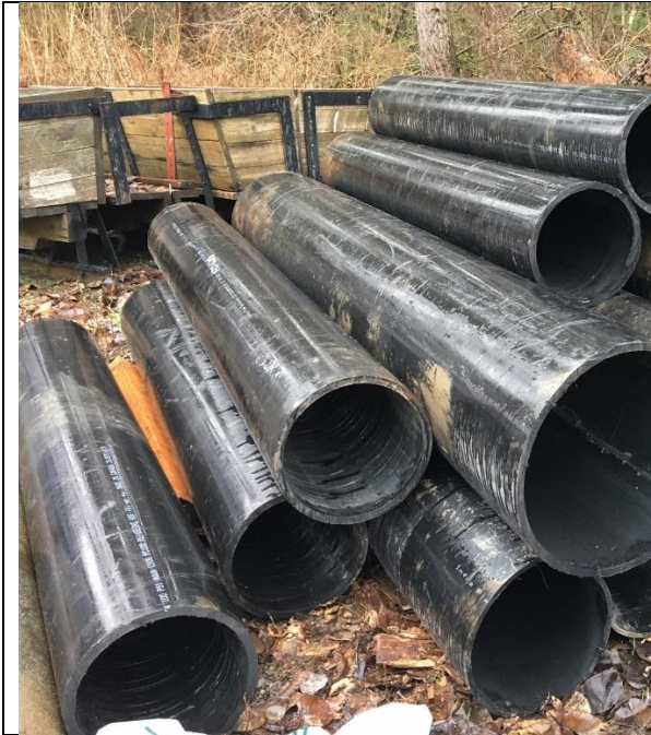
HDPE Water Main Pipe adapted for use as a trail culverts. Stockpile of inventory stored at the lagoon
